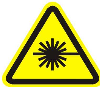
Laser Warning Symbol Located on front of laser above laser aperture, also internally on laser head assembly four places
